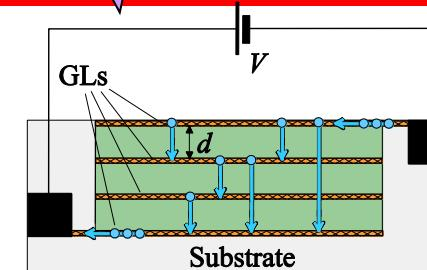
Hot-electron transistor with GL base as plasmonic THz detector
